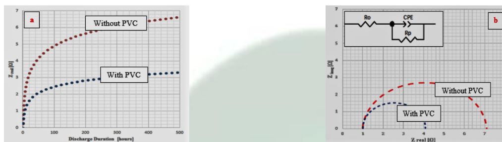
Figure 9 Impedance variation for cells with different electrolytes: (a) increase in internal resistance as a function of discharge time (b) nyquist diagram of ohmic resistance after complete discharge for PVC added Cell in comparison with PVC non-added Cell
