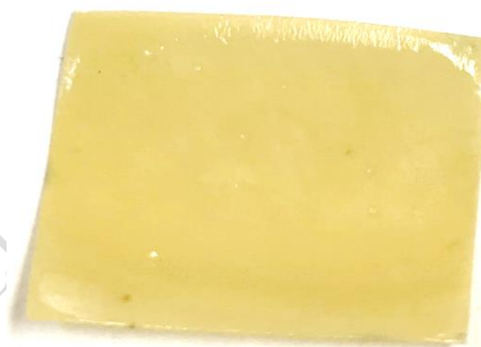
Fig 3. Prepared sulfonated polysulfone membrane with thickness of 110 \mu\text{m} .
